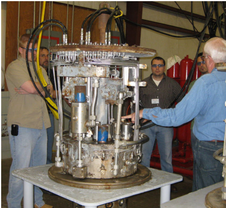
Subsea control pod
