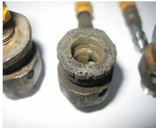
Figure 1: Schrader valve showing severe corrosion.
