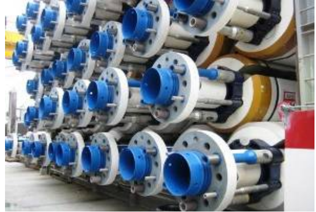
Figure 3: The risers have no protectors installed.
