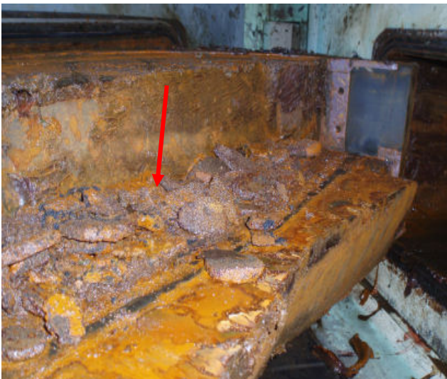
Figure 5: Red arrow shows caked blasting sand on the starboard blind shear ram block.
