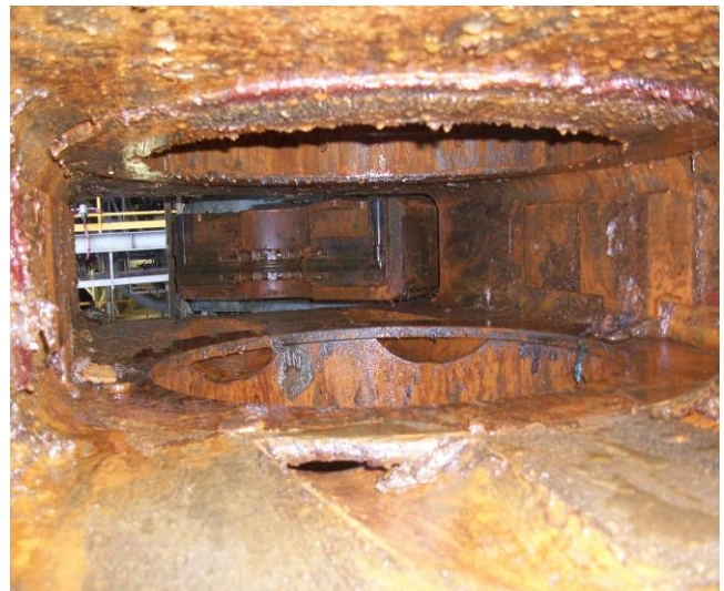
Figure 6: The red arrows show caked debris on the pipe ram's cavity.
