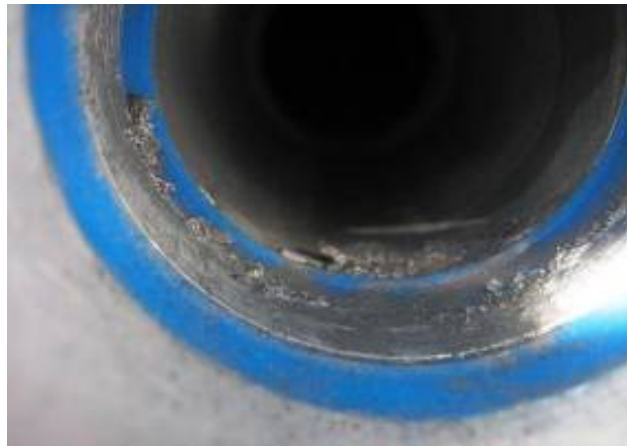
Figure 2: The hydraulic line box end has grit and an anti-seize material in the inner diameter.
