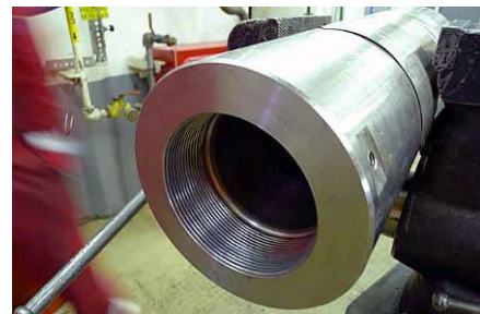
Accumulator body in vise after ejecting contents
