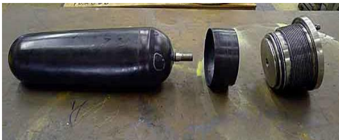
Bladder, internal molding and gas end cap ejected from accumulator
